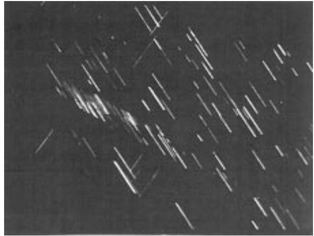
Figure 6 Typical DF micrograph of S' precipitates. Magnification \times 38000 .
